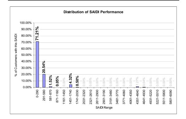
During the period 01/07/2010 to 30/06/2011 71% of customers experienced outages with durations of less than 290 minutes. Using a normalised data set this is increased to 83%.
